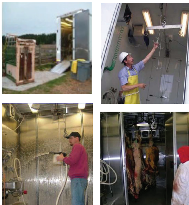
Figure 6. The general process of a mobile slaughter-type operation (clockwise from top left): Animals are restrained outside the unit and stunned; brought into the unit with a winch; the trailer door is closed, animals are minimally processed into halves and stored in the middle of the unit; the rear of the unit is cleaned, then the process begins again with the next animal.
