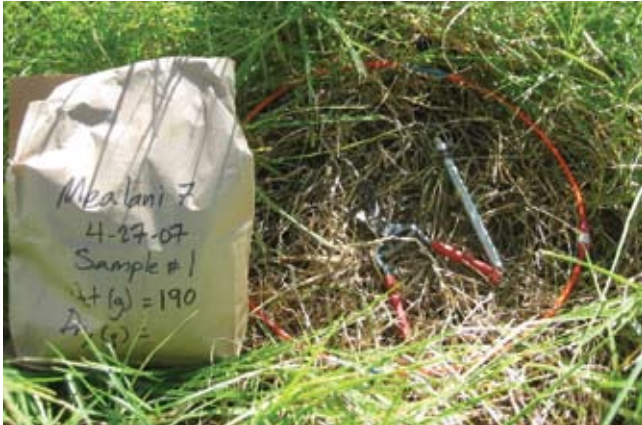
Figure 3. Simple tools such as a gram scale, clippers, paper bags, and a hoop of known area (a 1.2 sq ft area hoop is shown) are all that are needed to determine the amount of forage available for grazing.
