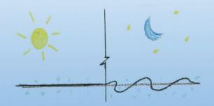
A typical problem that occurs is along hillsides when the expanding and contracting causes the pipe to creep down the hill making the top section of pipe straight and tight, and a pile of excess pipe at the bottom.
